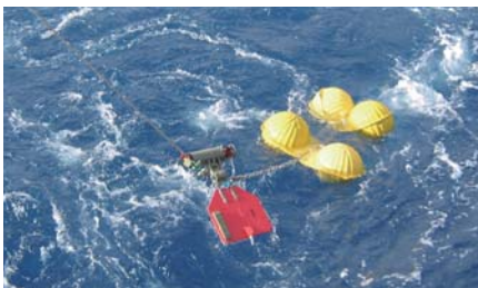
Deployment of the current meter
