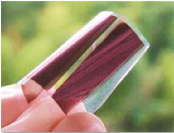
Solar cell made with transparent nanofiber paper
