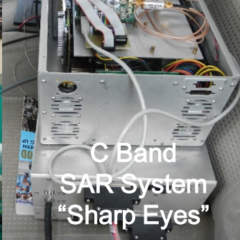
CP-SAR sensor development in clean room of Josaphat Laboratory
