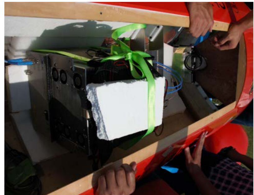
Installed CP-SAR sensor inside UAV JX-1 (below).
