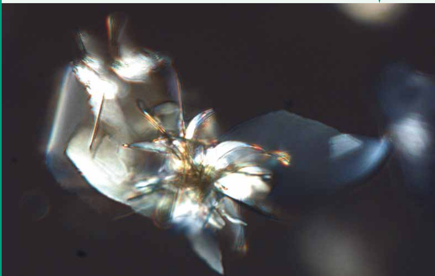
A crystalline assembly of azobenzene derivative and oleate showed oscillatory bending-unbending motion under continuous 435-nm light irradiation. The frequency of oscillation increased with increasing light intensity. (Ikegami T. et al., Angewandte Chemie International Edition , May 19, 2016)
