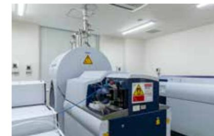
A mass spectrometry imaging system. It is characterized by its ability to simultaneously visualize a large variety of molecules by having a laser scan the surface of a tissue. It is used for analyses that are difficult for other imaging techniques to accomplish, including analyses of lipids and of the localization and structural changes of administered drugs (analyses of metabolites).
