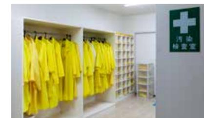
The contamination inspection room. To enter the controlled area, you must put on a special laboratory coat (a.k.a. a yellow coat) and footwear to prevent contamination. Before leaving the controlled area, you must measure your radiation exposure.
