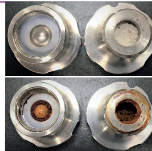
Reaction mixtures before and after grinding in a ball mill. Mechanoredox arylation reactions occurred with aryl diazonium salts and furan in the presence of a piezoelectric material (BaTiO<sub>3</sub>). (Kubota K. et al. *Science*, December 19, 2019)
