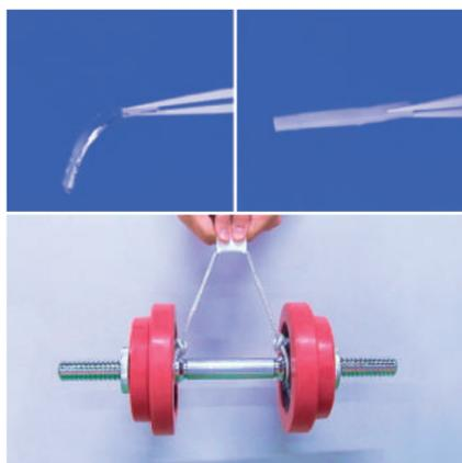
interactions between polymer molecules. This causes the material to rapidly transform from a soft, transparent hydrogel to a rigid, opaque plastic.
