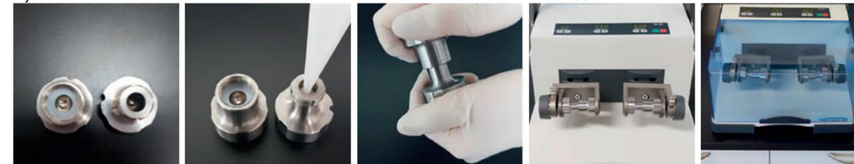
In ball milling, the chemicals and a steel ball are placed into steel jars which are then shaken vigorously.
