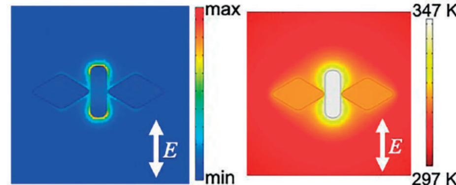
Calculated localized field (left) and temperature distribution (right) of the nano-butterfly structure. (Fujiwara H., et al, *Nano Letters*. December 23, 2019.)
