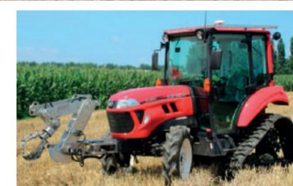
Equipment to harvest pumpkins attached to an unmanned tractor.
