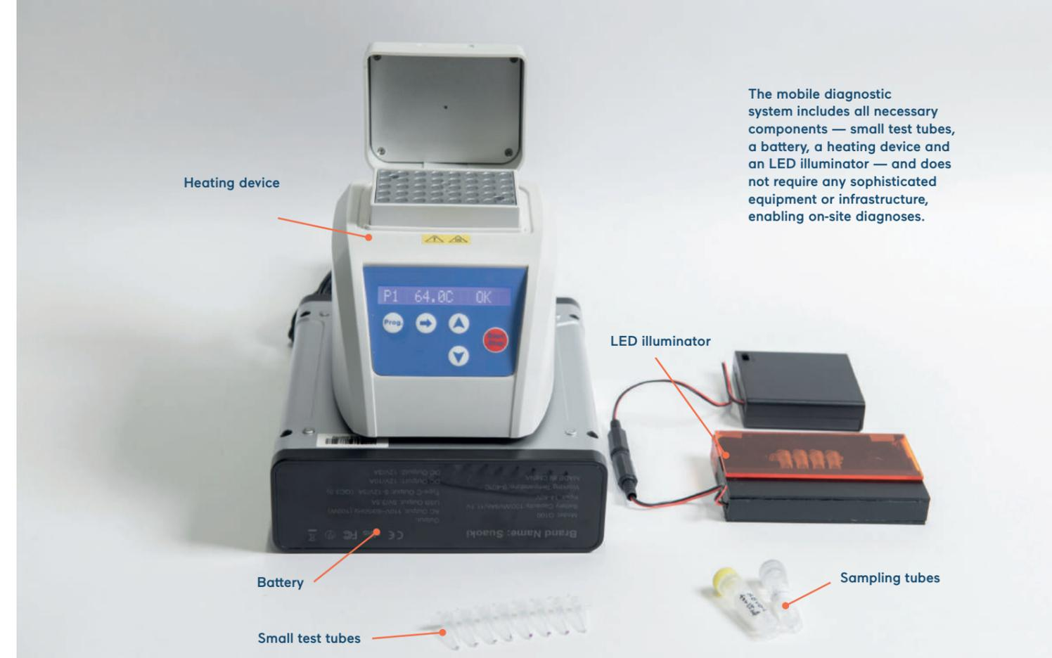
The mobile diagnostic system includes all necessary components — small test tubes, a battery, a heating device and an LED illuminator — and does not require any sophisticated equipment or infrastructure, enabling on-site diagnoses.
