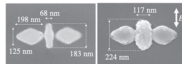
Scanning electron microscope images of the nano-butterfly structure before (left) and after (right) laser irradiation. Semiconductor zinc oxide has crystallized on the surface of the gold nanorod. (Fujiwara H., et al, *Nano Letters*. December 23, 2019.)
