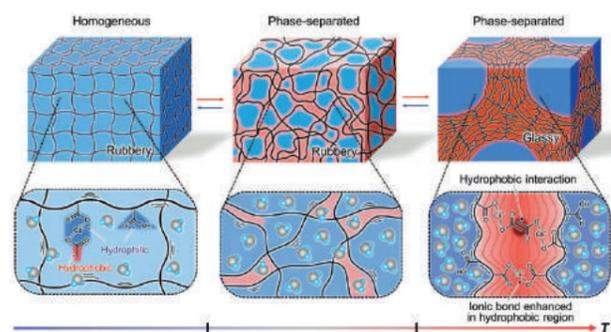
Molecular structures and the mechanisms behind instant thermal hardening of the hydrogel. (Nonoyama T. et al., *Advanced Materials*, November 18, 2019)
