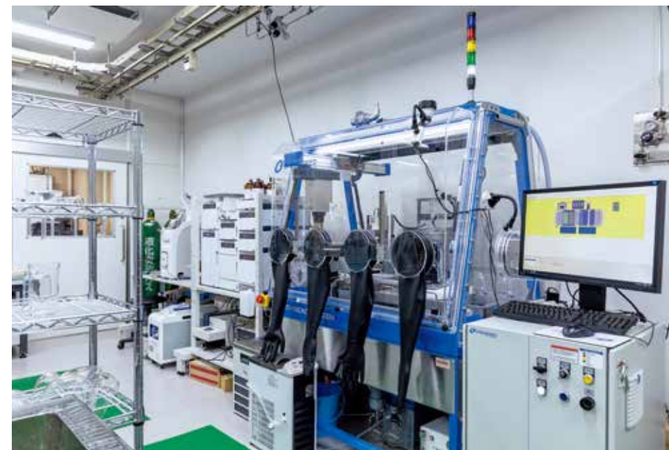
A synthesis workflow automation system manufactured by Chemspeed Technologies AG (a synthesis robot that can perform automated chemical reactions).
