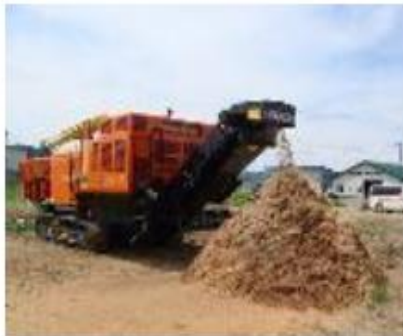
Shredder machine manufacturing woody materials
