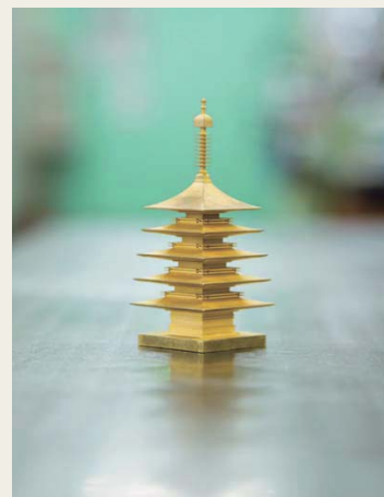
A five-story pagoda measuring five centimeters in height created by cutting brass using a wire electric discharge machine. This is an artistic sample created by the Machining Solution Division.
