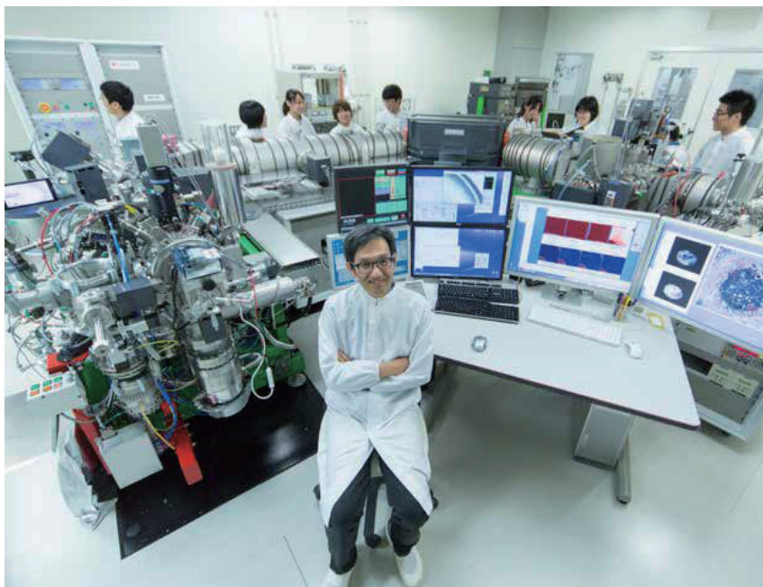
Professor Yurimoto and the isotope microscope system developed at his laboratory (2015 photo).
