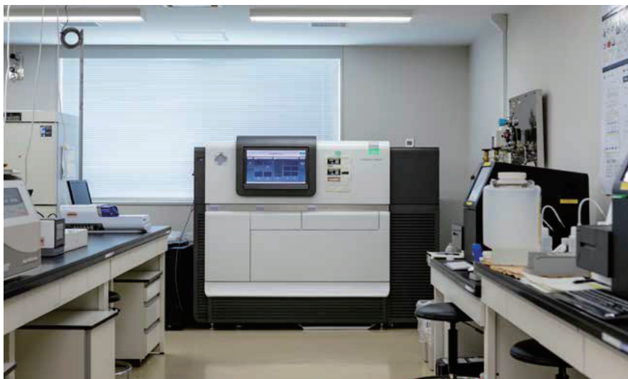
This next-generation sequencer allows large amounts of genetic data to be gathered within a short time, enabling the early detection of novel viruses.
