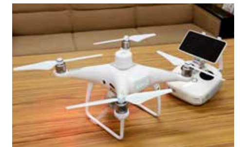
UAV used for disaster investigation and research: Phantom 4 RTK of DJI Co., Ltd. By communicating with a base station in real time, aerial photo data with location information can be obtained and high-precision topographical data can be created.
