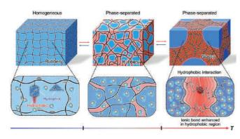
Molecular structures and the mechanisms behind instant thermal hardening of the hydrogel. (Nonoyama T. et al., Advanced Materials, November 18, 2019)
