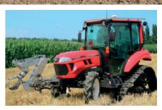
Equipment to harvest pumpkins attached to an unmanned tractor
