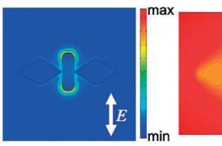
Calculated localized field (left) and temperature distribution (right) of the nano-butterfly structure. (Fujiwara H., et al, Nano Letters. December 23, 2019.)
