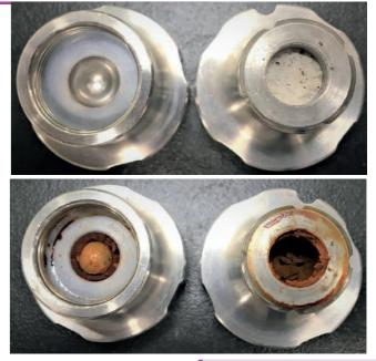
Reaction mixtures before and after grinding in a ball mill. Mechanoredox arylation reactions occurred with aryl diazonium salts and furan in the presence of a piezoelectric material (BaTiO3). (Kubota K. et al. *Science*, December 19, 2019)
