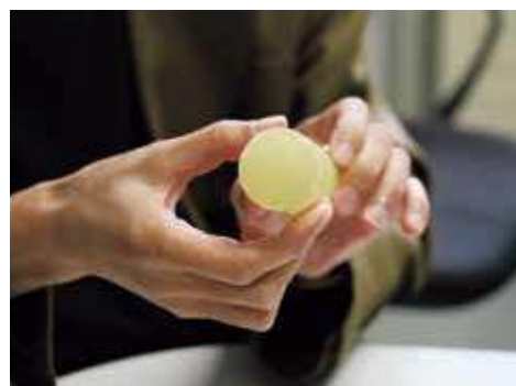
Perforated plastic used as fuel for hybrid rockets
